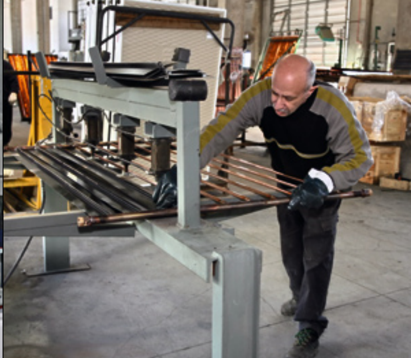
Absorber manufacturing: An Amcor employee solders an absorber tube.
