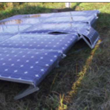
Gone with the wind: In January of 2007, the windstorm called Kyrill greatly increased the number of damage reports that insurance firms received in Europe related to PV systems.
