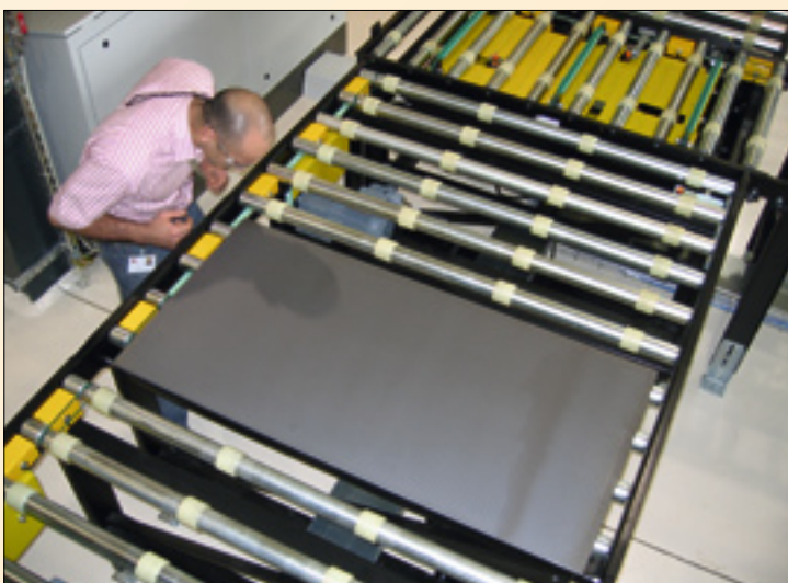
Critical eye over the finished product: a cadmium telluride module of First Solar, USA
