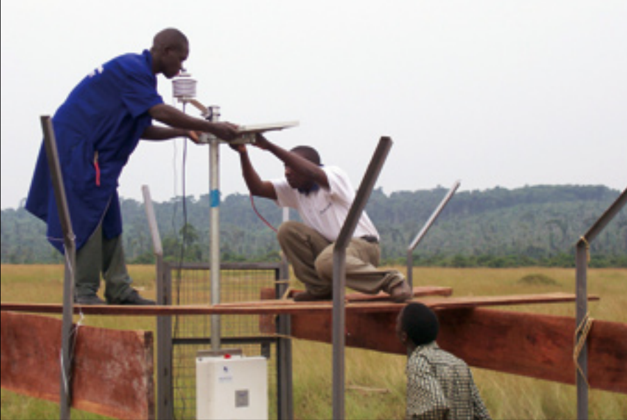
Renewable education at work: Jagwe Wycliff from Uganda, one of the former PPRE students, installed several pyranometers to determine the global solar radiation in his home country.
